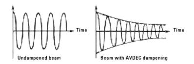
AVDEC damping material is composed of a layer of visco-elastic material sandwiched between two layers of metal. It converts vibrational energy into heat energy by shear deformation of the visco-elastic layer, resulting in a significan reduction in sound and vibration levels.
